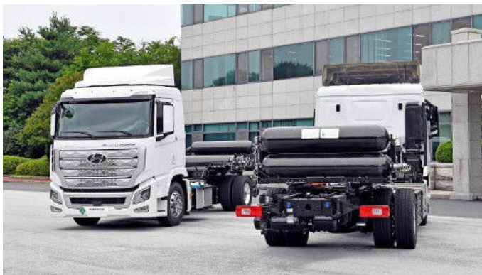
Fig. 5.21: left: XCIENT fuel cell truck (Hyundai); right: GenH 2 with LH 2 tanks of Daimler Trucks (Daimler Trucks)
