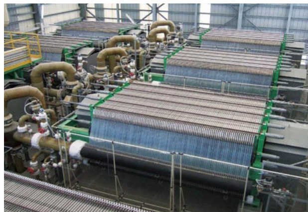
Fig. 5.13: Typical large scale electrolyser set-up (Thyssen-Krupp 7 )
